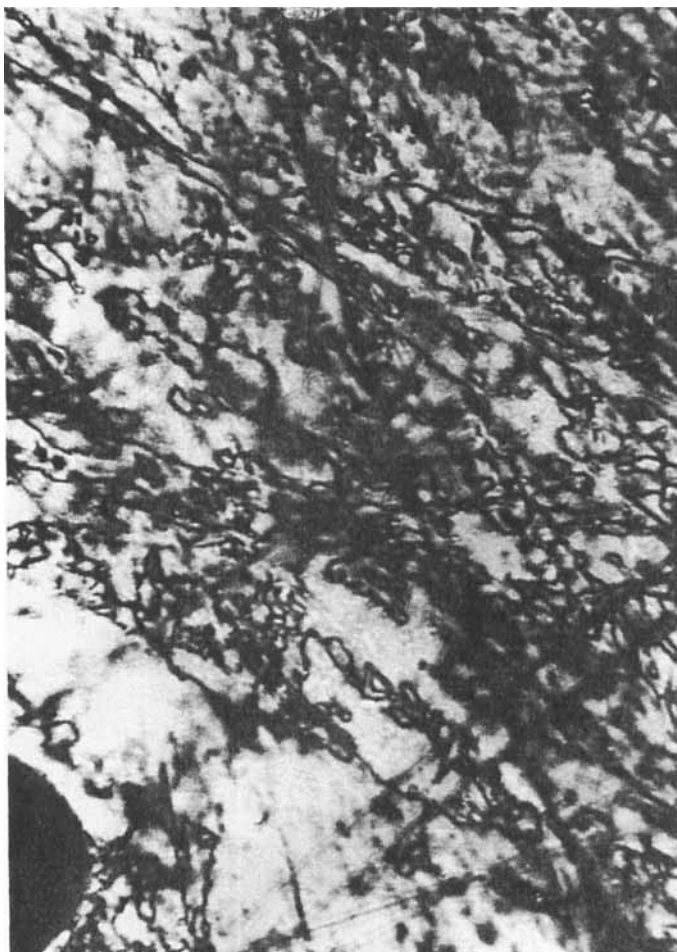
FIGURE 7 b) Nematic phase. T = 380 K on cooling. Crossed polarizers.
