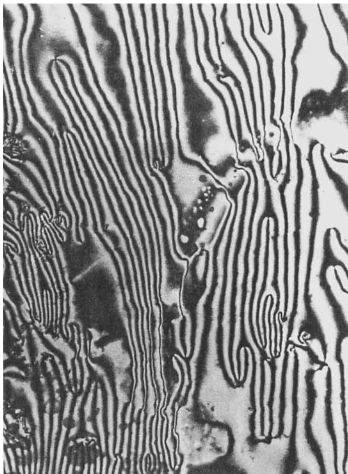
FIGURE 5 b) Schlieren texture, domain pattern induced by shearing; covered layer. T = 391 K. Crossed polarizers.
